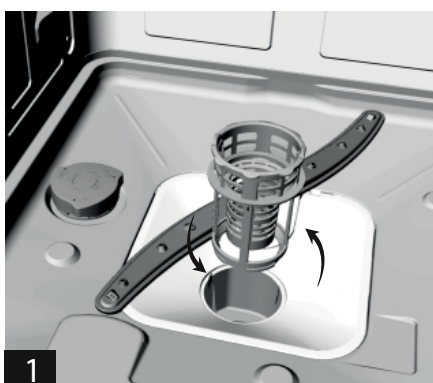
Korak 1: Filter zasučite proti smeri urnega kazalca in ga izvlecite.
